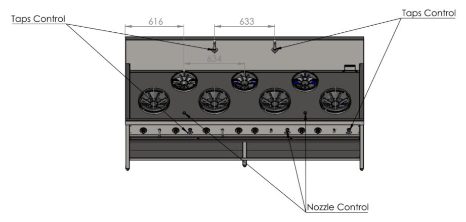
Note: 2 Nozzles controlled by single valve 2 Taps 2 valves
