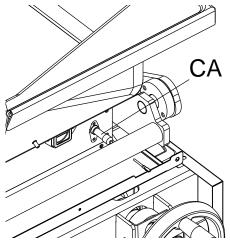
To replace the detection electrode, remove the left side, loosen the fixing screws and remove the components.
