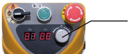
Set the speed control to the desired speed by rotating speed button clockwise to raise speed, counterclockwise to lower speed.
