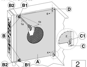
To refit the suction wall, repeat the steps in reverse order and retighten nut C1.
