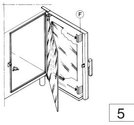
After cleaning close the internal panel ensuring it is properly seated against the rubber stops.
