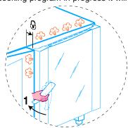
b) Turn the handle all the way counter-clockwise to open the oven door fully.
