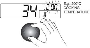
Turn the knob clockwise (to increase the value) or counter clockwise (to decrease the value) to set the desired COOKING TEMPERATURE in the small DISPLAY.
