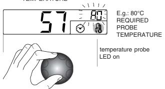
Turn the knob clockwise (to increase the value) or counter clockwise (to decrease the value) to set the DESIRED PROBE TEMPERATURE on the small DISPLAY.
