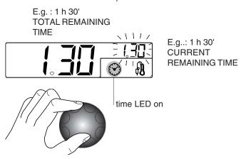
Turn the knob clockwise (to increase the value) or counter clockwise (to decrease the value) to set the desired cooking TIME on the small DISPLAY.
