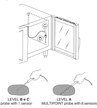
The LEVEL **A** oven is equipped with a MULTIPOINT probe with 6 sensors located at intervals along the wand, enabling the correct temperature to be read in the centre of the product even if the probe tip is not positioned at the product core. Close the oven door.
